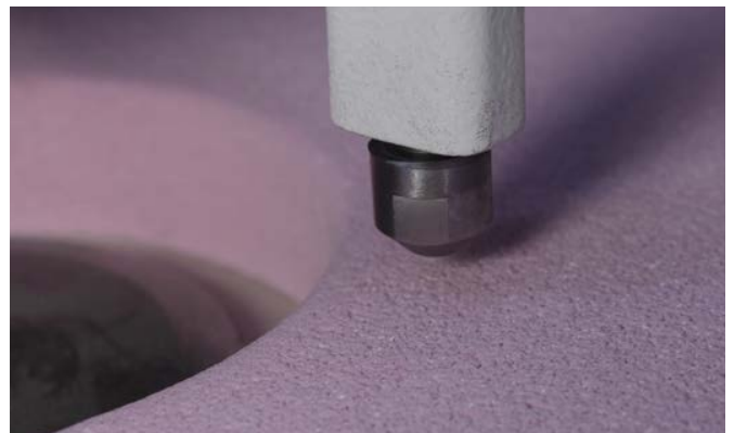
Automatic dressing of the grinding stone
