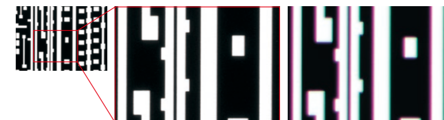
Apochromat optics (captured with SMZ1270+P-Plan Apo 1x/WF)
