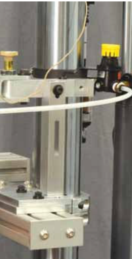
High temperature Low-Cycle Fatigue (LCF) test setup.
