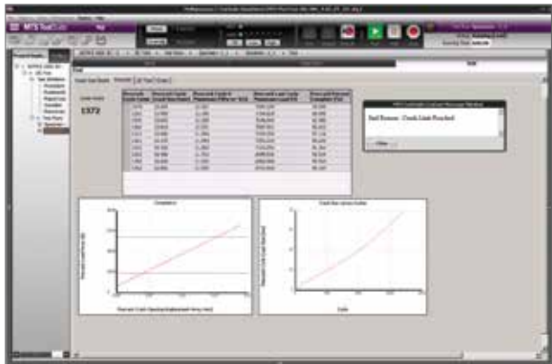
The Runtime View of the pre-crack portion of the JIc test displays tabular results per cycle, load versus COD, and crack size versus cycles.
