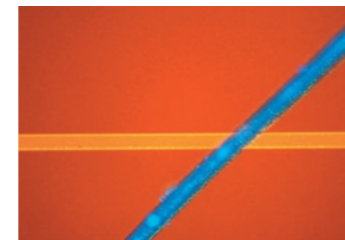
Epi-fluorescence observation of organic substance on wafer
